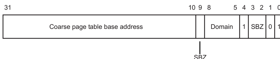
Figure 7-6 Coarse page table descriptor
